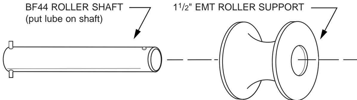
**Works with BT12515 1 1/2" EMT shoe on Mechanical Sidewinder Bender.**
