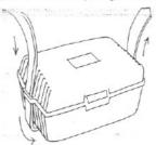
Pass the strap DOWN through the first case lug, under the case and UP through the other lug.
