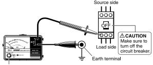
(2) Check the circuit under test is not energized as follows. Connect the test leads to the circuit under test and read a voltage
